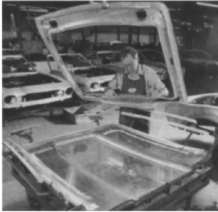
Fig. 36.13 A structural adhesive used to bond a stiffener to an aluminum car bonnet. To line up the two parts a purpose made fixture is designed.
