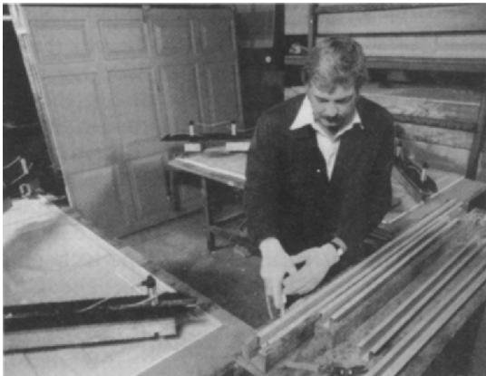
Fig. 36.14 Mild steel stiffeners are bonded to up and over garage door. Result: rigidity; unblemished exterior surfaces.
